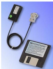
The interface converter is provided with a one meter long connection cable which can be directly inserted into the COM port of PC. The humidity-temperature sensor is connected at the 6-pin female western connector (RJ12).
