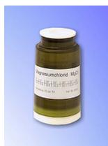
The accuracy possible under stable temperature environment conditions is in the range of 1 % relative humidity. The working principle is based on a saturated salt solution, over which a specific relative humidity value
